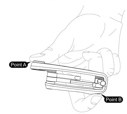
• T25 can be moved to the torque-enabled end of the tool, by swapping the T25 with the 4mm hex key.
